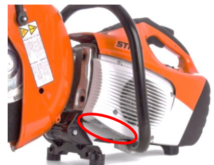
Serial number location on some current disc cutters.
